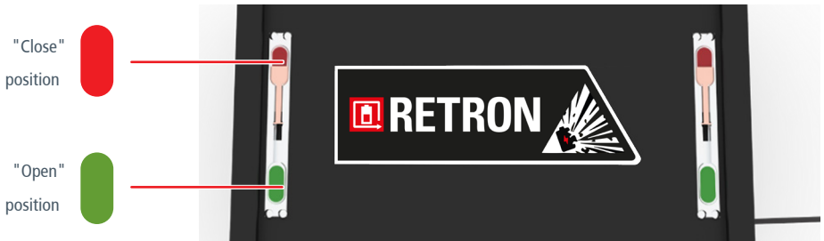
Fig. 2 Locking lever in "closed" position
